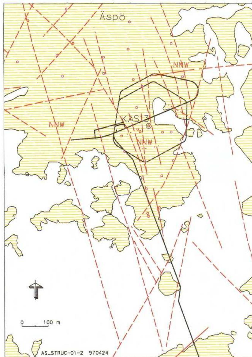
**Figure 2-2.** Minor fracture zone interpretation in the Äspö area based on pre-investigation data. Surface map. /Gustafson et al, 1991/.
