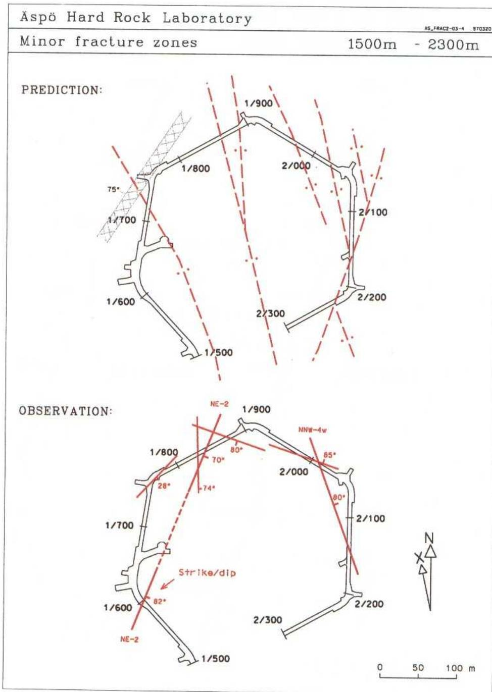
**Figure 2-5.** Comparison between the minor fracture zone prediction (based on pre-investigation data) and outcome (based on tunnel data). Chainage 1500-2300 m. Note, that features mapped as 'fractures' (less than 10 cm wide) are not included.
