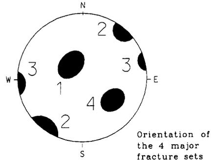
**Figure 2-8.** Structural models on the (50-m) block scale. Small scale fracturing. Fracture network model for rock blocks P50-03 and P50-04 based on tunnel data.
