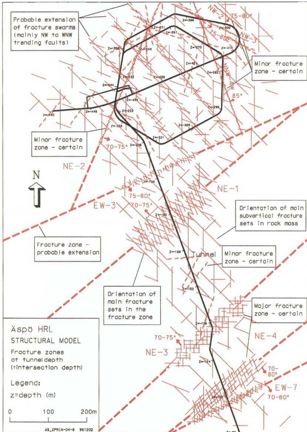
**Figure 2-11.** Structural model of the rock mass surrounding the Äspö tunnel. The model represents the positions and estimated extents of fracture zones (swarms) at tunnel level. The orientation of the main subvertical fracture sets in major fracture zones and the intact rock mass are based on tunnel mapping data. 'Fracture swarms' comprise concentrations of subparallel, often water-bearing faults.
