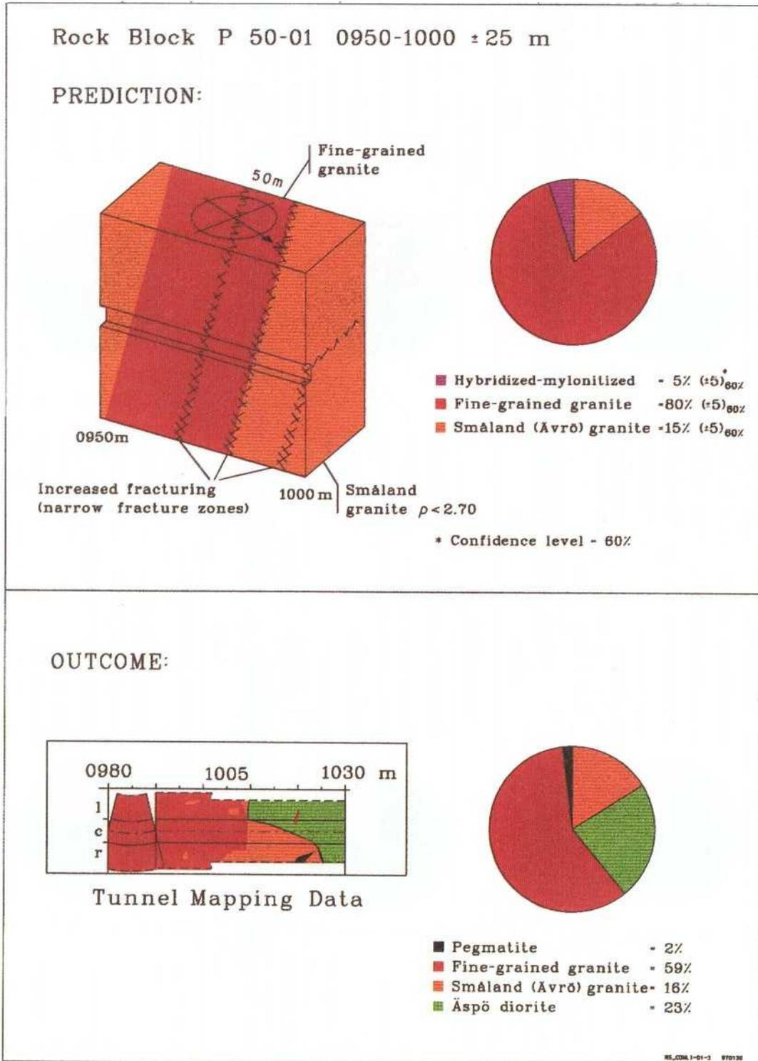
Figure 3-4. Comparison between the prediction and outcome on the (50-m) block scale. Lithological model. P50-01.
