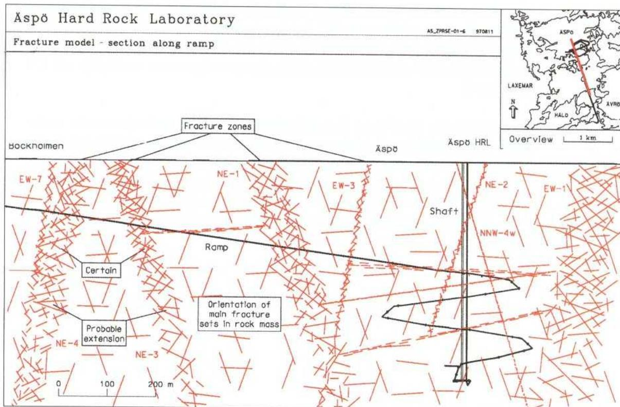
*Figure 2-12. Structural model - section along ramp.*
