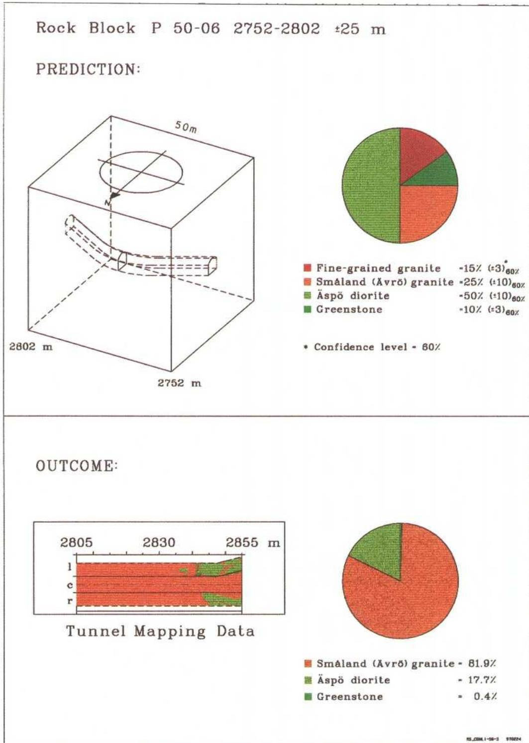
Figure 3-9. Comparison between the prediction and outcome on the (50-m) block scale. Lithological model. P50-06.
