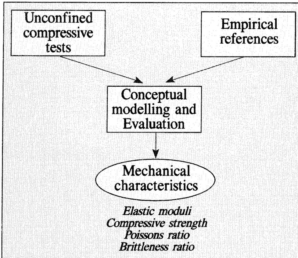
*Figure 3-1. Flow chart of the mechanical characteristics programme.*
