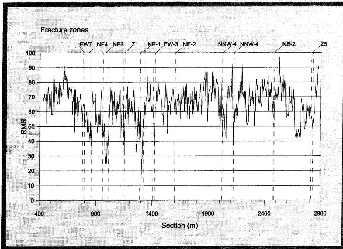
*Figure 1-3. Observed RMR values along the tunnel /Stille-Olsson, 1996/.*
