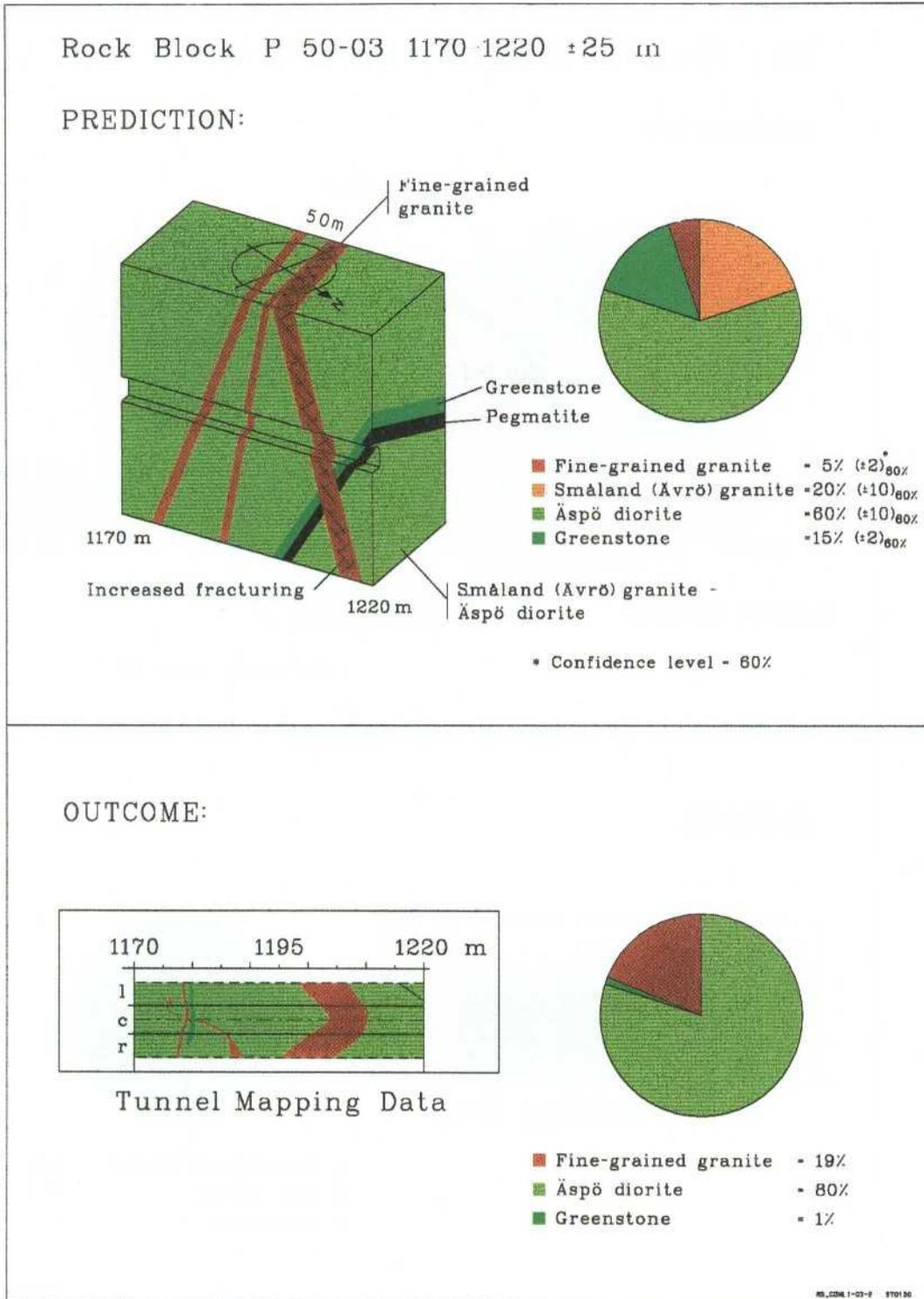
**Figure 3-6.** Comparison between the prediction and outcome on the (50-m) block scale. Lithological model. P50-03.
