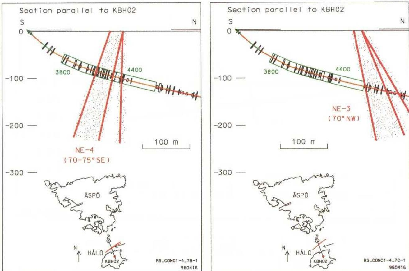
**Figure 1-4.** Fracture zones NE-3 and NE-4. Prediction. /According to Gustafson et al, 1991/.
