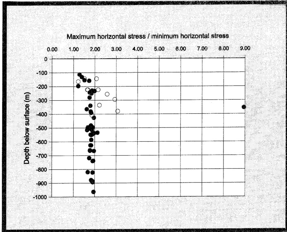
*Figure 2-4. Ratio between the highest and lowest horizontal stress /Stille-Olsson, 1996/.*
