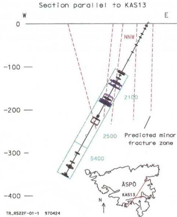
**Figure 2-3.** Interpretation of the minor fracture zone system 'NNW' in a section parallel to borehole KAS13 based on pre-investigation data /Wikberg et al, 1991/.
