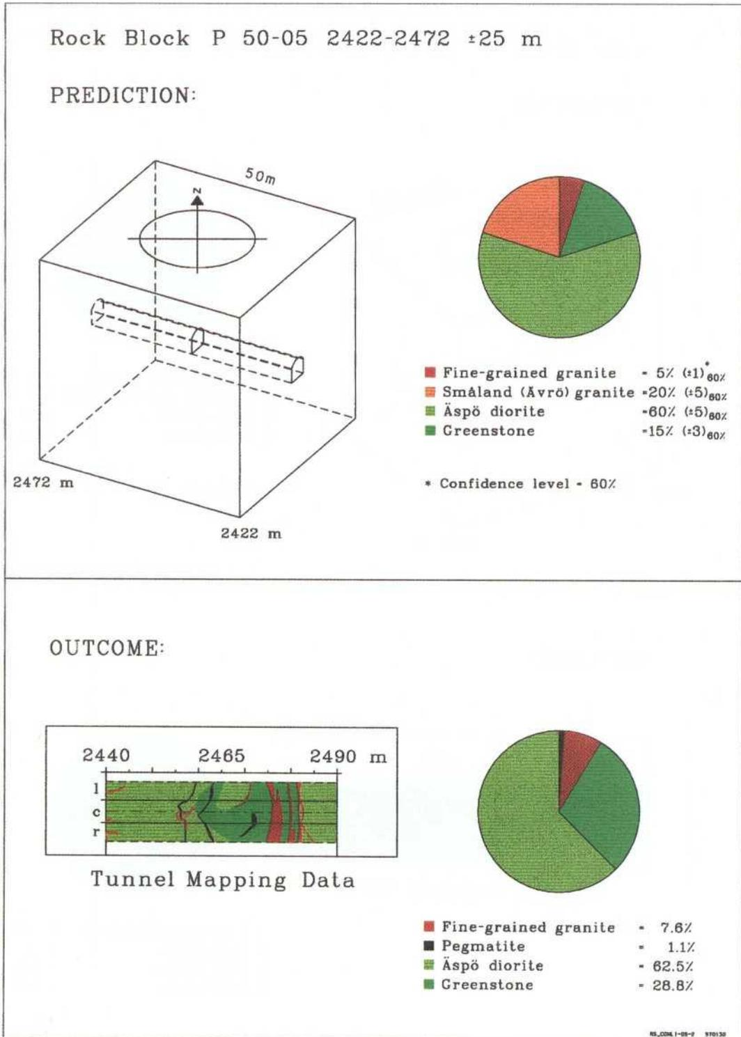
Figure 3-8. Comparison between the prediction and outcome on the (50-m) block scale. Lithological model. P50-05.
