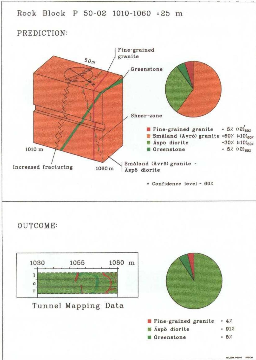
Figure 3-5. Comparison between the prediction and outcome on the (50-m) block scale. Lithological model. P50-02.
