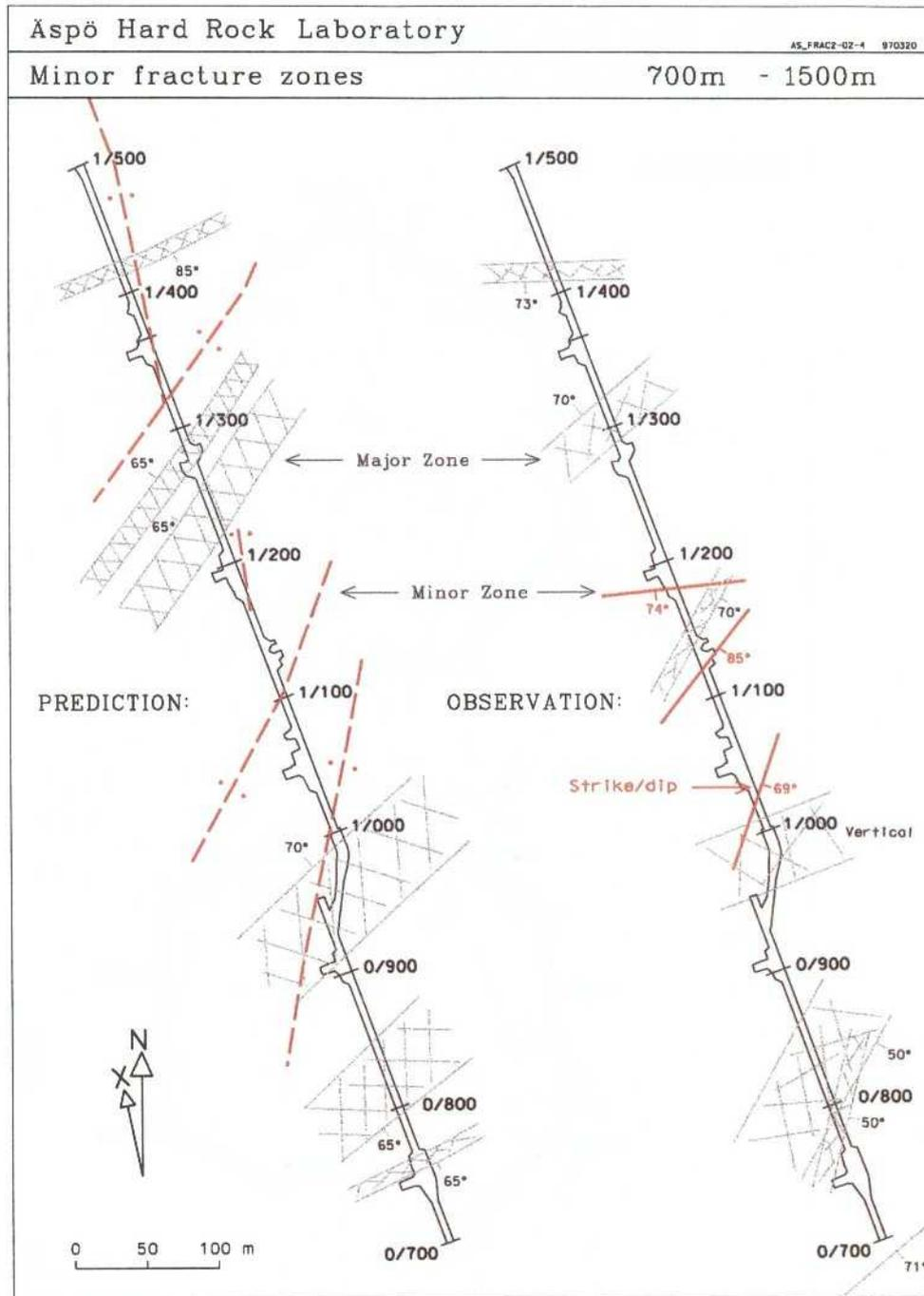
**Figure 2-4.** Comparison between the minor fracture zone prediction (based on pre-investigation data) and outcome (based on tunnel data). Chainage 700-1500 m. Note, that features mapped as 'fractures' (less than 10 cm wide) are not included.
