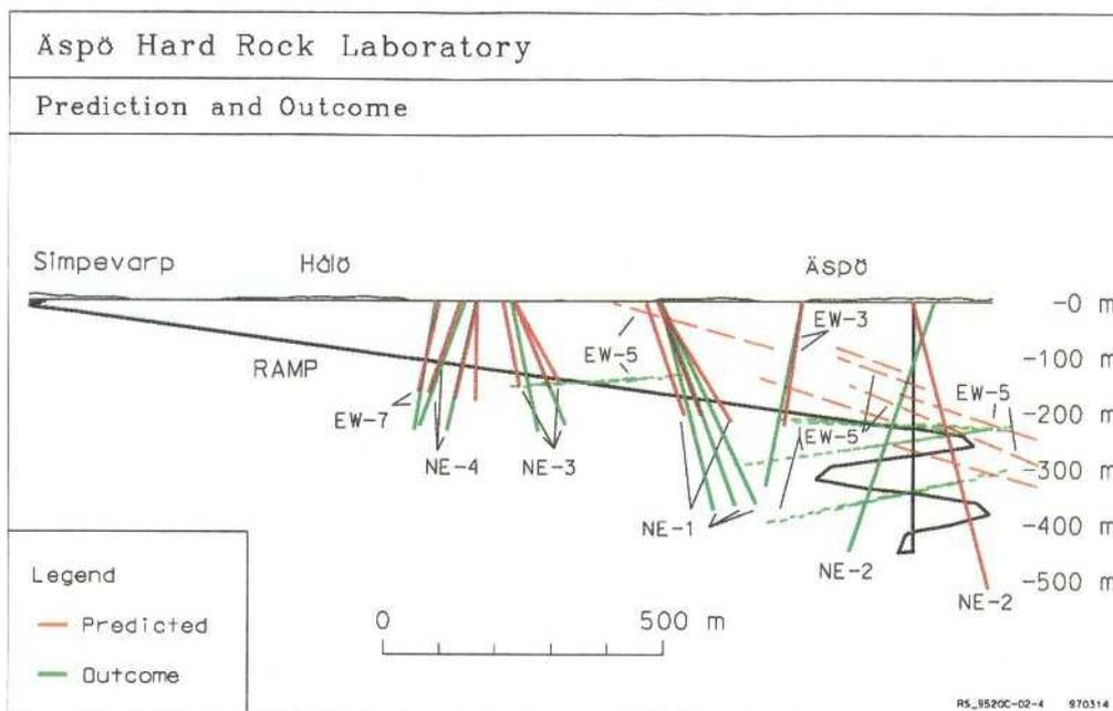
**Figure 1.** Prediction and outcome for major fracture zones. The picture illustrates predicted (red) and observed (green) positions and dips in the tunnel.
