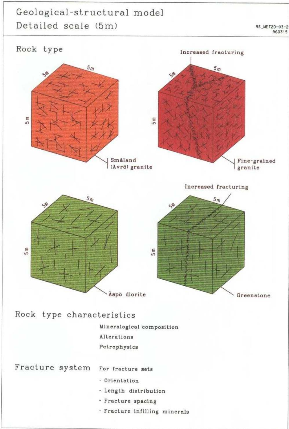
**Figure 3-11** Overview of the subject rock type characteristics of the lithological models (for the four main rock types), addressed on the detailed scale.
