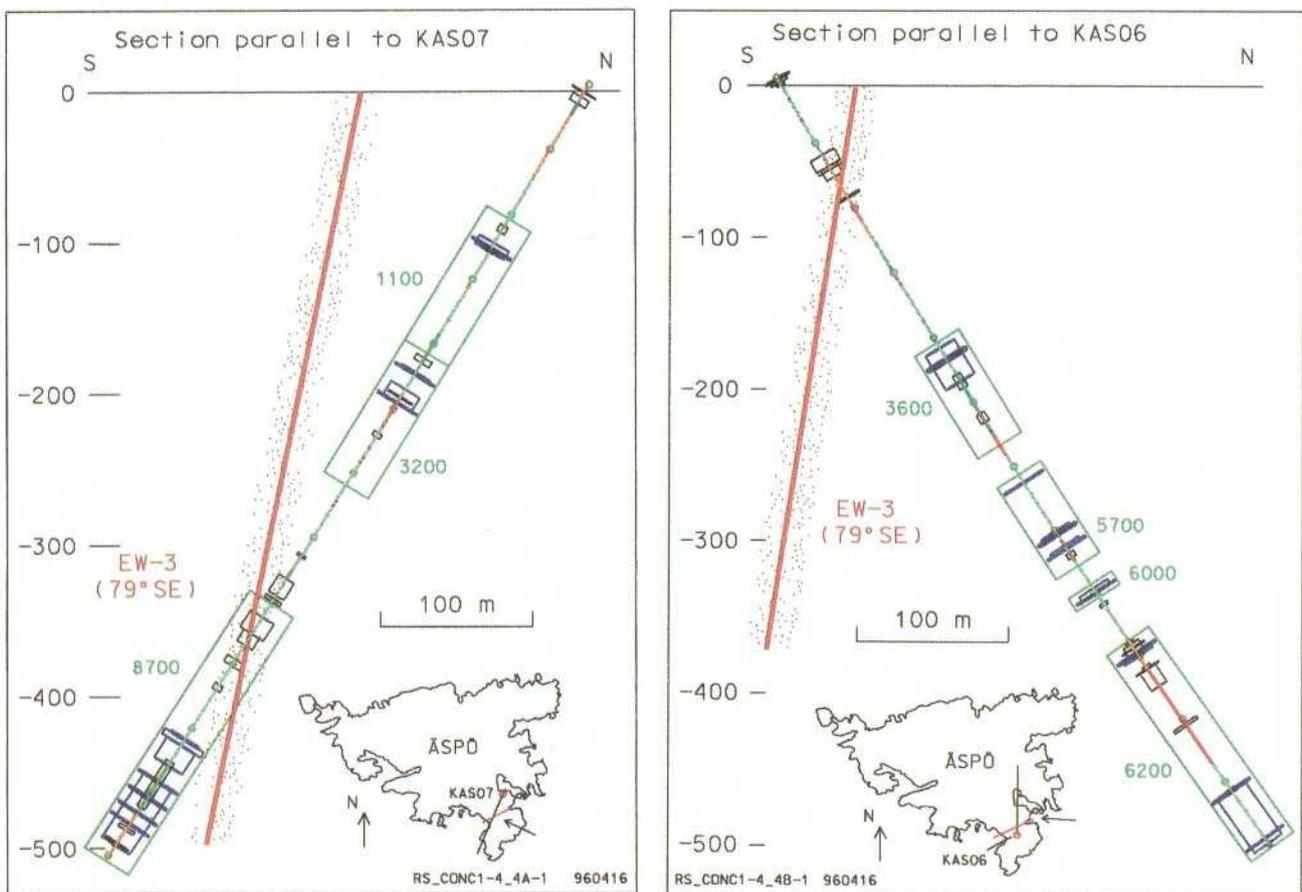
**Figure 1-10. Fracture zone EW-3. Prediction. /According to Gustafson et al, 1991/.**
