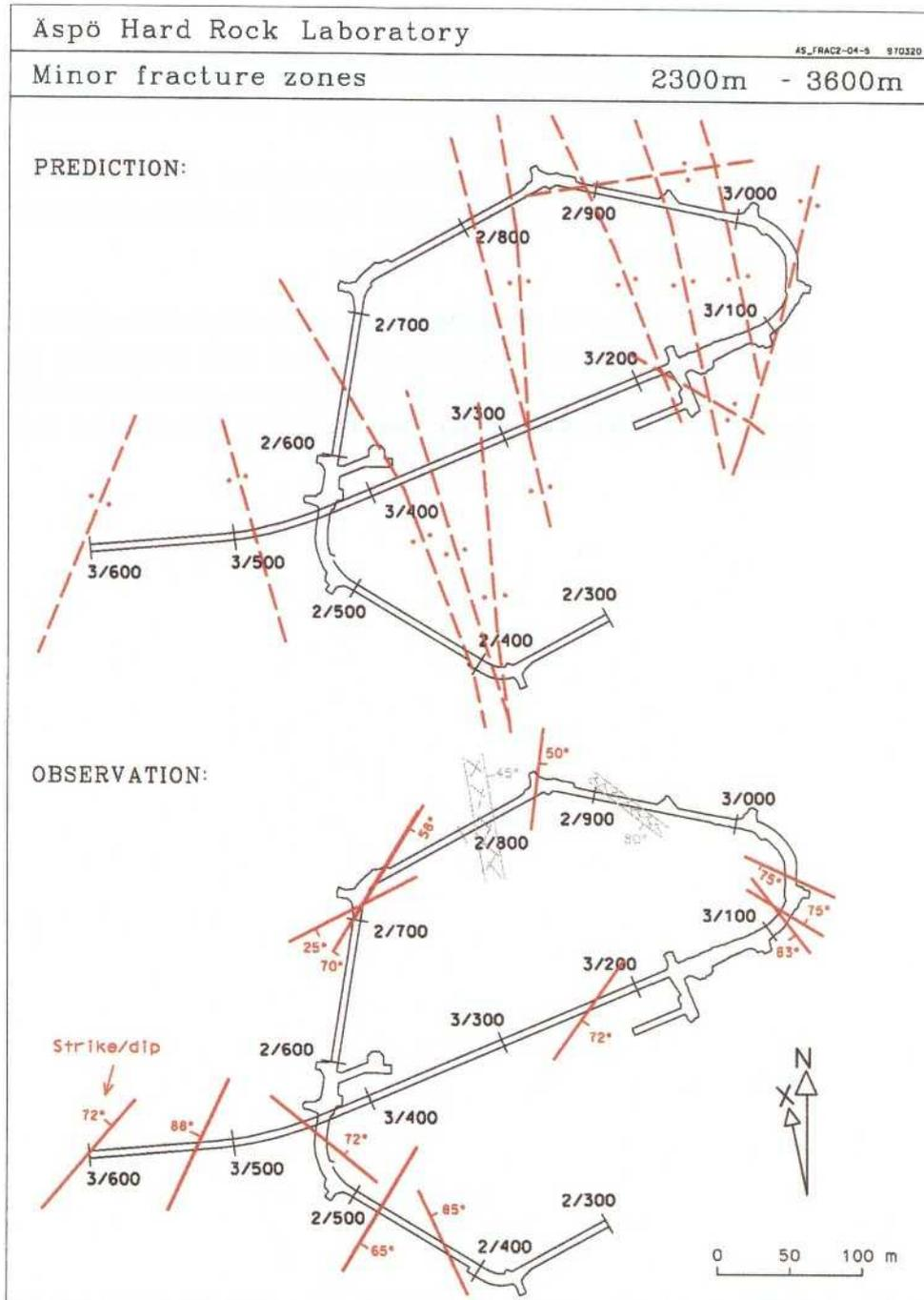
**Figure 2-6.** Comparison between the minor fracture zone prediction (based on pre-investigation data) and outcome (based on tunnel data). Chainage 2300-3600 m. Note, that features mapped as 'fractures' (less than 10 cm wide) are not included.
