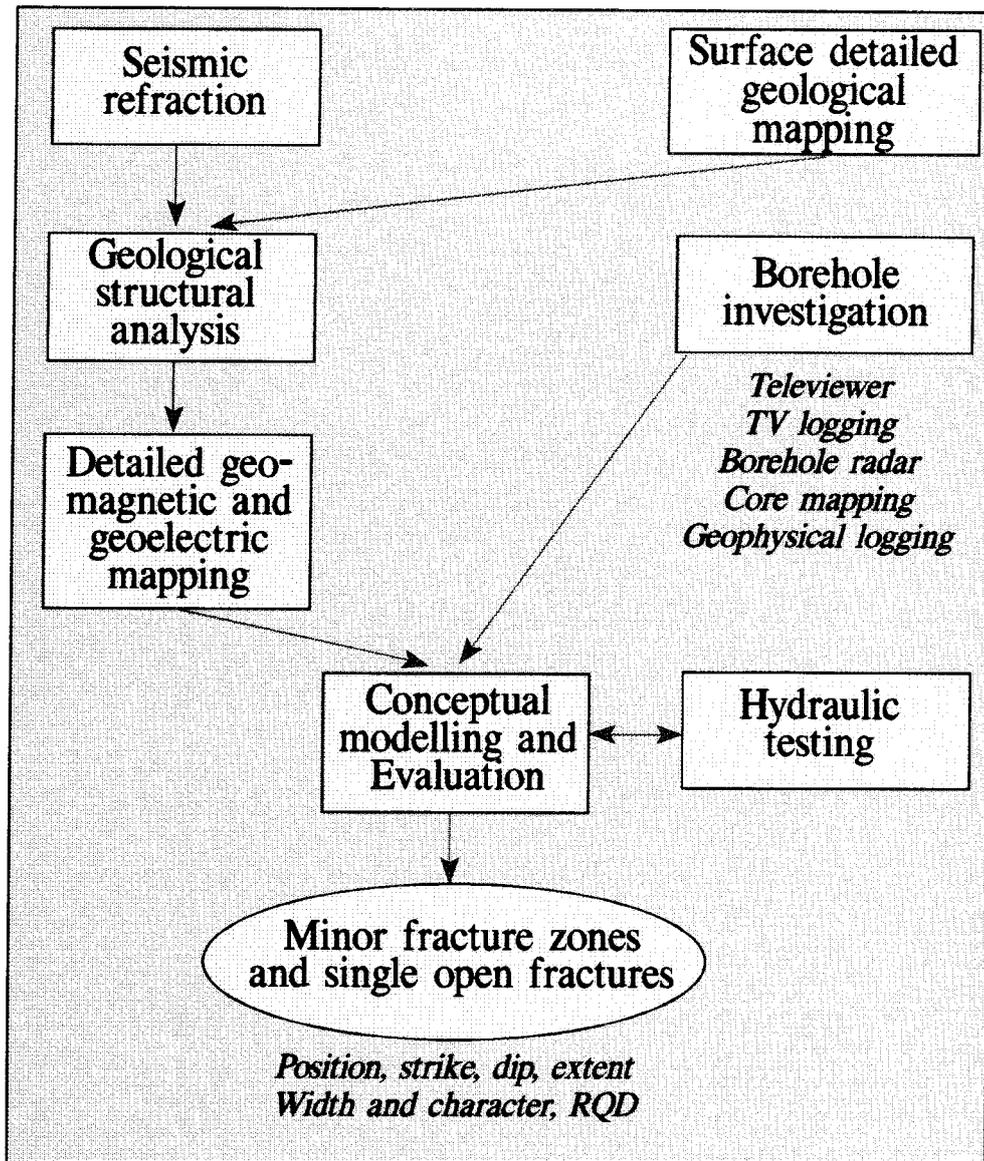
*Figure 2-1. Pre-investigation methodology. Structural-geological characterization. Minor fracture zones, single open fractures and small-scale fracturing.*
