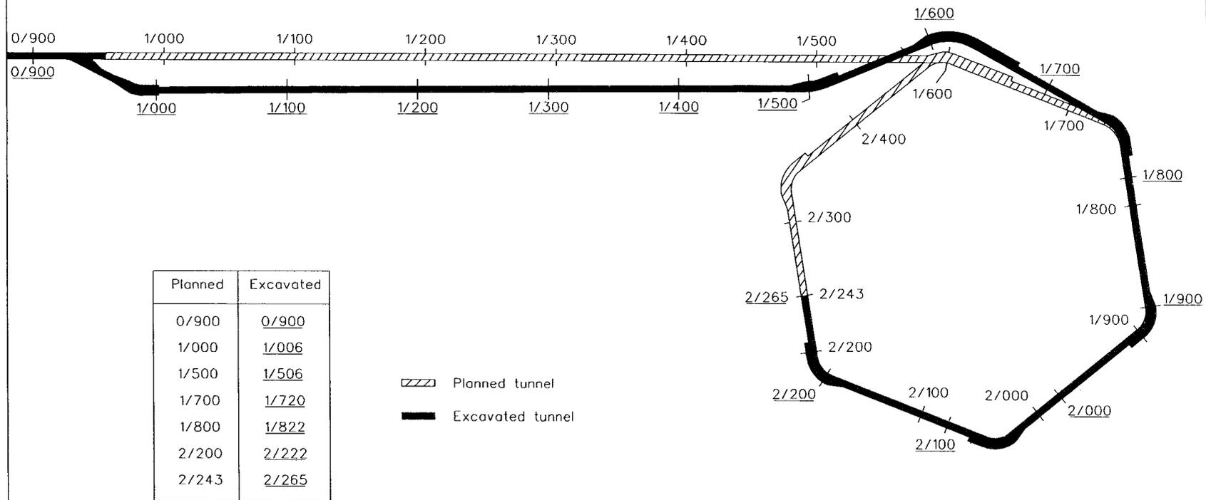
Figure I-5. The planned and excavated tunnel layouts.
