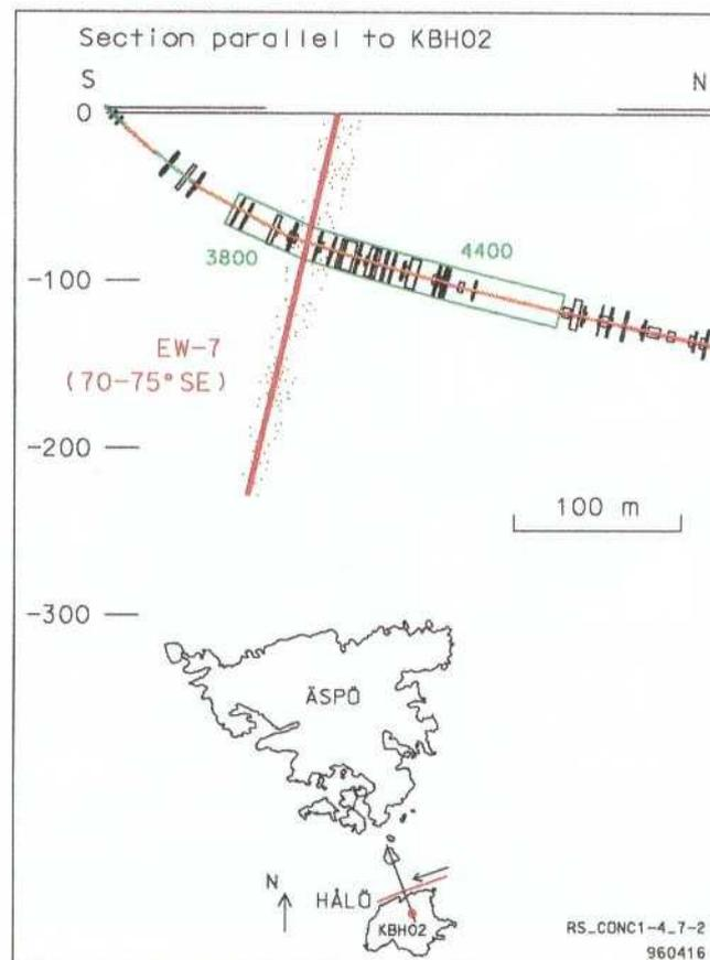
**Figure 1-2.** Fracture zone EW-7. Prediction. /According to Gustafson et al, 1991/.
