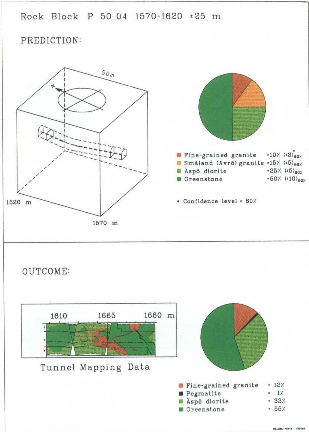
**Figure 3-7.** Comparison between the prediction and outcome on the (50-m) block scale. Lithological model. P50-04.
