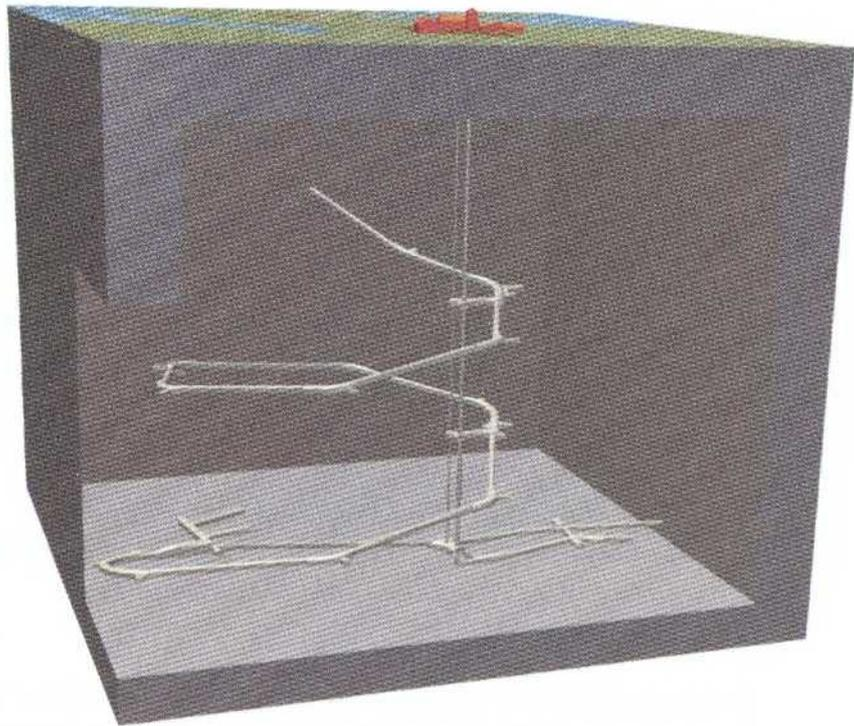
*Figure I-3. General layout of the Äspö HRL. The total length of the tunnel is 3600 m. The first part of the tunnel was excavated using the drill-and-blast technique. The last 400 metres were excavated by a Tunnel Boring Machine (TBM) with a diameter of 5 metres. The underground excavations are connected to the Äspö Research Village, containing offices, stores, hoist and ventilation building, by a hoist shaft and two ventilation shafts.*
