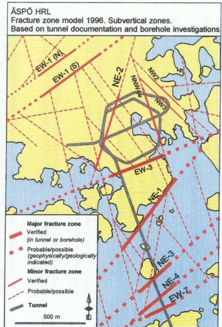
Figure 2. Structural model of the Äspö area, with predicted main structures at ground level, prior to construction (left) and after construction (right).
