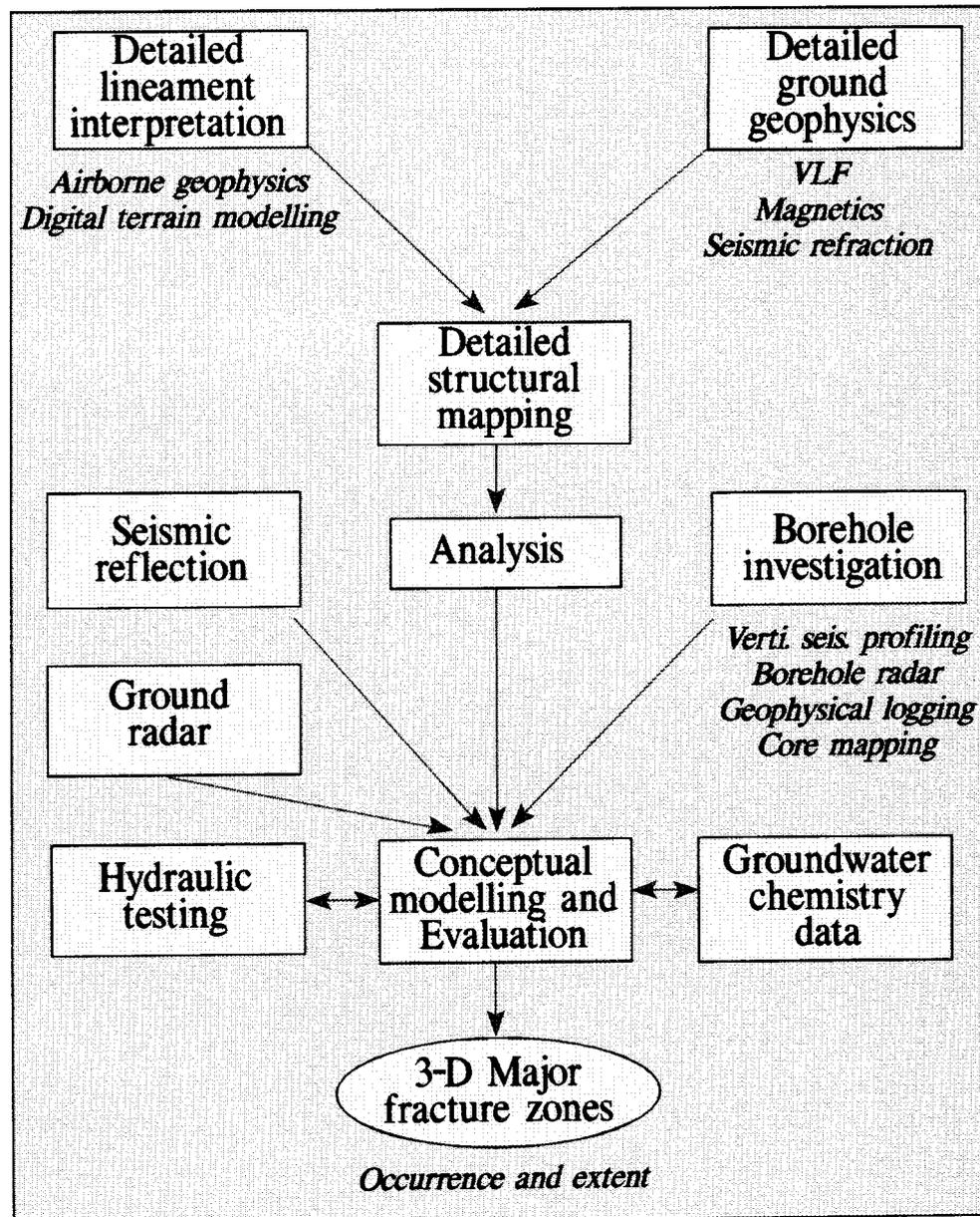
**Figure 1-1.** Pre-investigation methodology. Structural-geological characterization. Major fracture zones.
