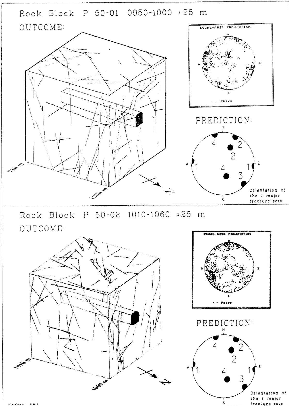
*Figure 2-7. Structural models on the (50-m) block scale. Small scale fracturing. Fracture network model made for rock blocks P50-01 and P50-02 based on tunnel data.*
