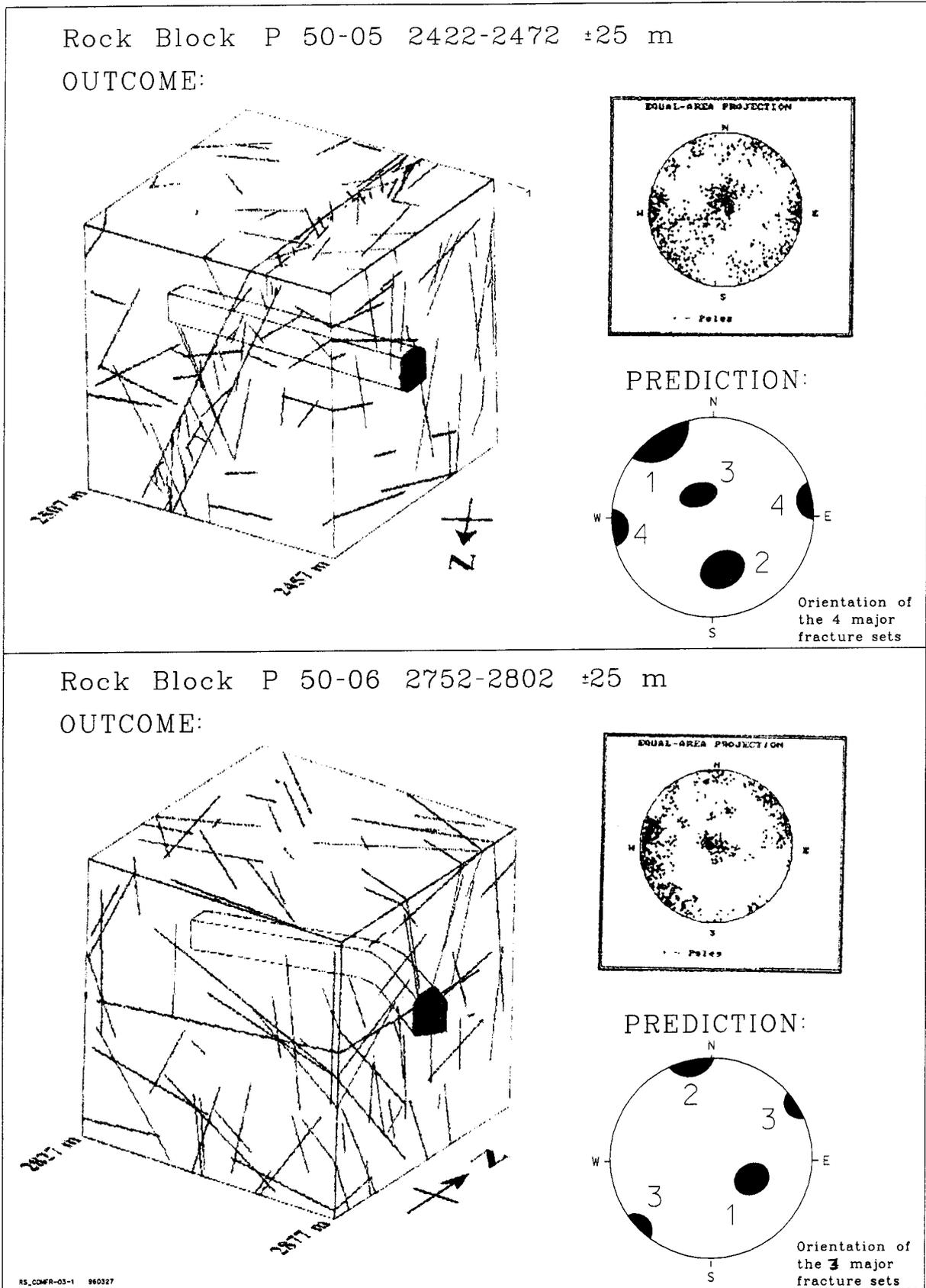
**Figure 2-9.** Structural models on the (50-m) block scale. Small scale fracturing. Fracture network model for rock blocks P50-05 and P50-06 based on tunnel data.
