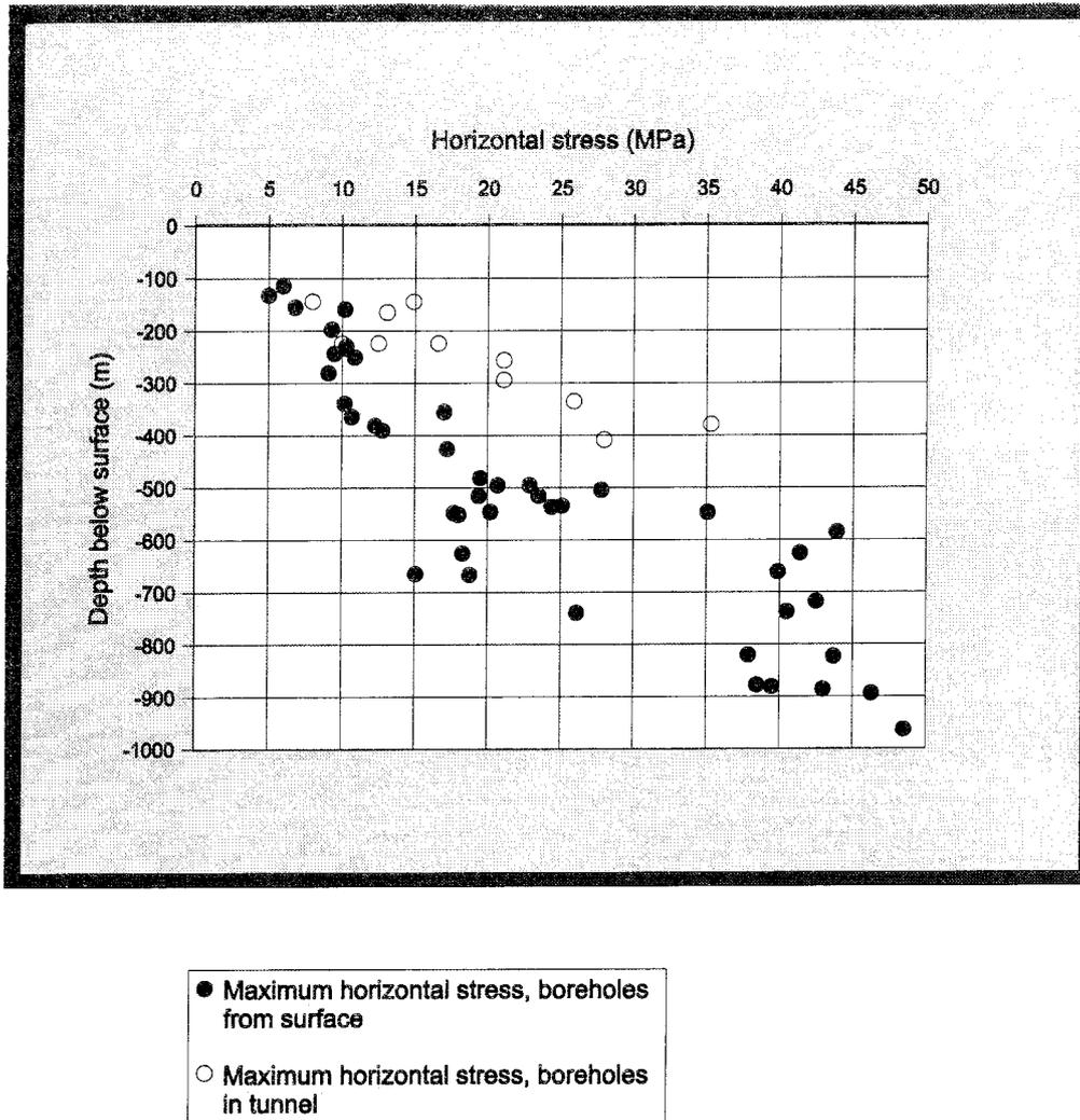
*Figure 2-3. Measured maximum horizontal stress /Stille-Olsson, 1996/.*
